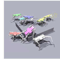
Figure 4: A performance benchmark of skills learned in the obstacle navigation task, where the SMODICE-expert is initialized in front of a box of height 0.2m and reaches a target position behind the box. The learned skills exhibit diverse behaviors that cover various modalities of the offline dataset.
